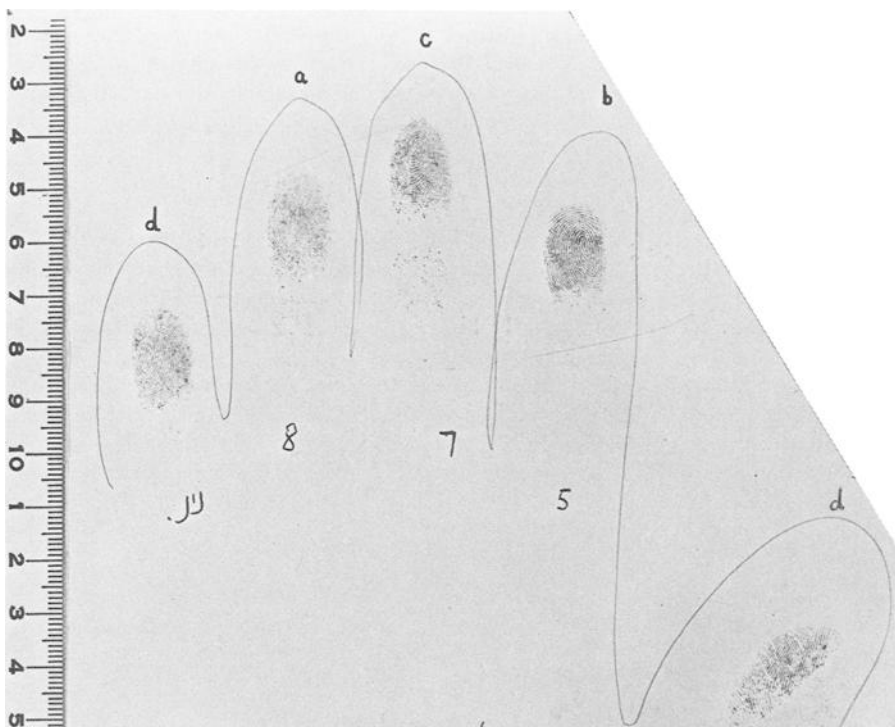
FIG. 3—Impressions of six-week-old latent fingerprints from a good donor obtained with the ninhydrin analogues: (a) Compound II; (b) Compound III; (c) Compound IV; and (d) ninhydrin.
